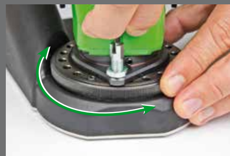
Depth adjustment (0.1 - 1.0 mm)
