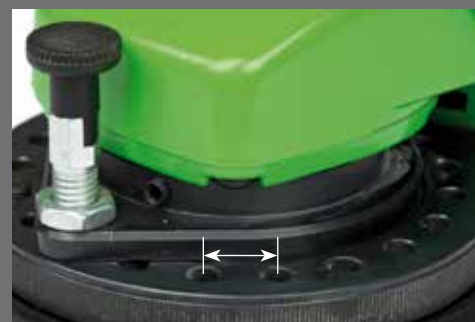
one detent corresponds to a depth of 0.1 mm
