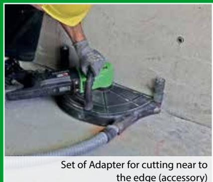
Set of Adapter for cutting near to the edge (accessory)
