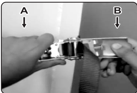
Hold clamp A & tighten the belt by adjusting clamp B. Stop the locking when securely tighten the belt.
