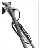
Wind the line cord of the tool on the holder meant for this purpose. Make sure that the switch of the floor guiding device is not pressed or locked. Plug the grinder in the socket of the floor guiding device. Lead the hose of the vacuum cleaner above the floor guiding device, connect it with the grinder. The clamp will avoid a slipping of the hose.
