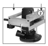
Put the top frame with the weights 2 on the frame handle of the machine
