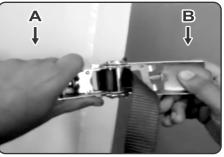
Hold clamp A & tighten the belt by adjusting clamp B.
