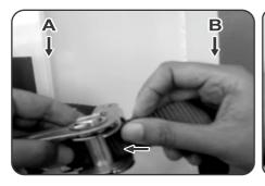
Hold clamp A by left hand insert the belt through slot provided on calmp shaft.
