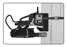
Now magnetic core drill is ready for vertical / overhead drilling application.
