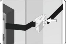
Insert the belt through clamping slot.
