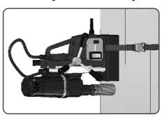
ALWAYS USE THE SAFETY BELT WHEN USING MAGNETIC CORE DRILL VERTICALLY OR UP-SIDE DOWN POSITION.
