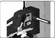
Pass the safety belt through the opening provided in the body.
