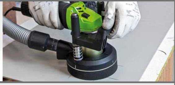
Exact positioning of the machine due to the support hood & LED-light
