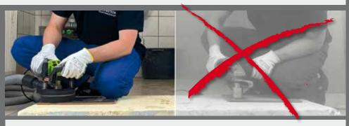
Due to dust exhaust best **protection of the user against dangerous mineral dusts,** compared to conventional methods with angle grinders
