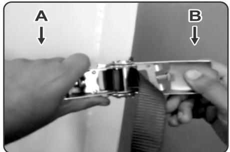
Hold clamp A & tighten the belt by adjusting clamp B.
